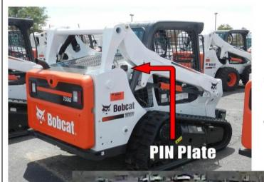
Pictured is a similar Bobcat T-590. The machine PIN plate is on the right side of the upper frame, just rearward of the cab and inset from the loader arm.
