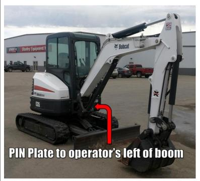
Pictured is an example image of an E-35. The PIN plate is on the lower front, to the operator's left of the boom.
